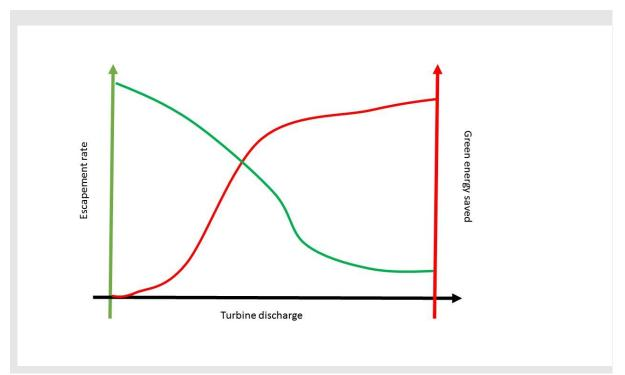
*Figure 12 : Schematic representation of the evolution of the turbine escapement rate and the proportion of green energy saved as a function of the turbined flow at a hydroelectric structure.*
