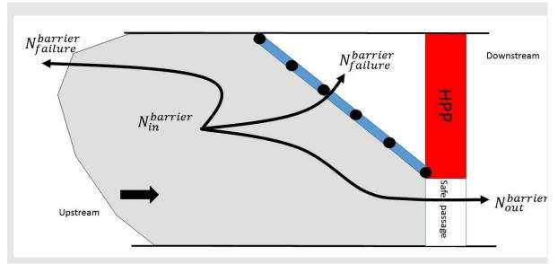
Figure 11 : Efficiency measurement of a surface behavioral barrier.
