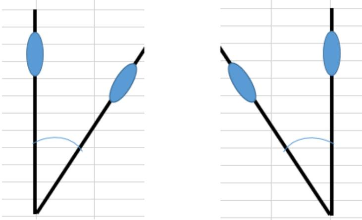
Electrodes lying down for trashes passage    Electrodes standing up again after trashes passage
