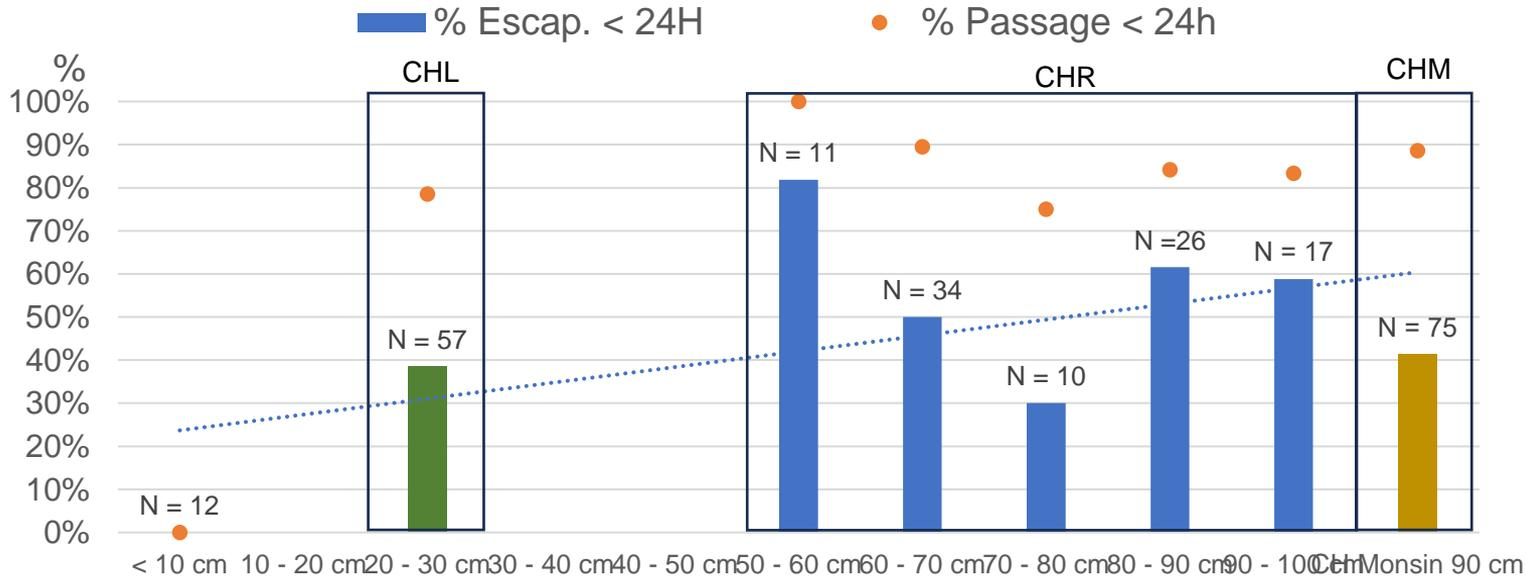
CHL : close to 40% efficiency with 20-30 cm of gate opening (close to the HPP)
